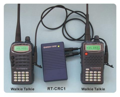
This picture just shows the connection of Receiver, Repeater Controller and Transmitter. For real repeater system, the antennas of both receiver and transmitter maybe extended and installed for approximate 10 meters, or use a DUPLEXER to combine the RF signal of receiver and transmitter. These are the ways to provide adequate rejection of strong transmitter signal occurring at the receiving signal.
